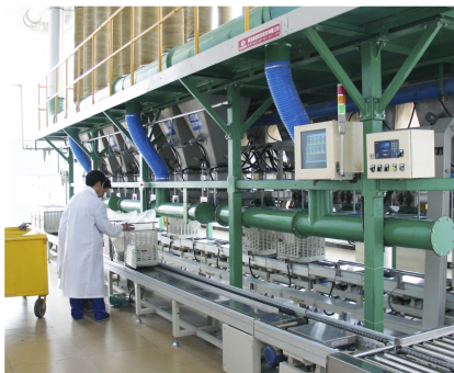
1. Automatic chemical powder weighing system for mixer
