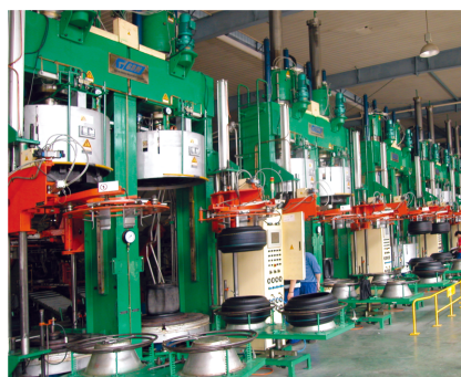
6. Steel-belted radial tyre hydraulic dual-mould curing press
