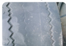
Tread Wear Under High Air Pressure
