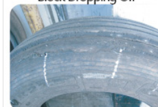
Shoulder Damage & Pattern Block Dropping Off
