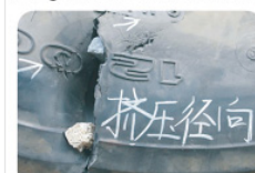
Foreign Material Between Side Wall
