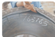
Puncture and Delamination
